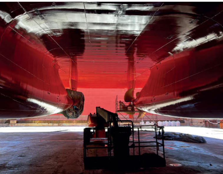
THE VISENTINI MK II BOASTS A TOTALLY NEW HULL DESIGN WITH FULL TWIN SKEGS. SOURCE: CAPTAIN PHILIPPE SILLAN
