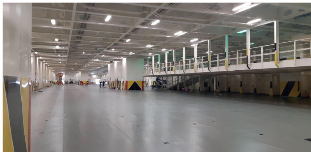
THE FULLY ENCLOSED 983LM UPPER VEHICLE DECK HAS A FIXED CAR DECK ON THE PORTSIDE FORWARD. SOURCE: CAPTAIN PHILIPPE SILLAN
