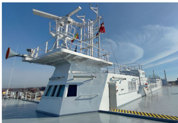
AS PER SRTP STIPULATIONS, AURA SEAWAYS IS EQUIPPED WITH A SECOND BRIDGE
