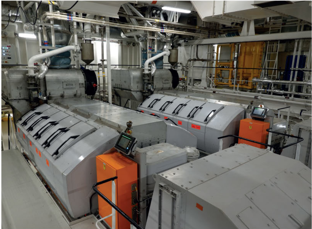
TWO OF THE SIX WÄRTSILÄ W10V31DF FOUR-STROKE ENGINES. SOURCE: PHILIPPE HOLTHOF
