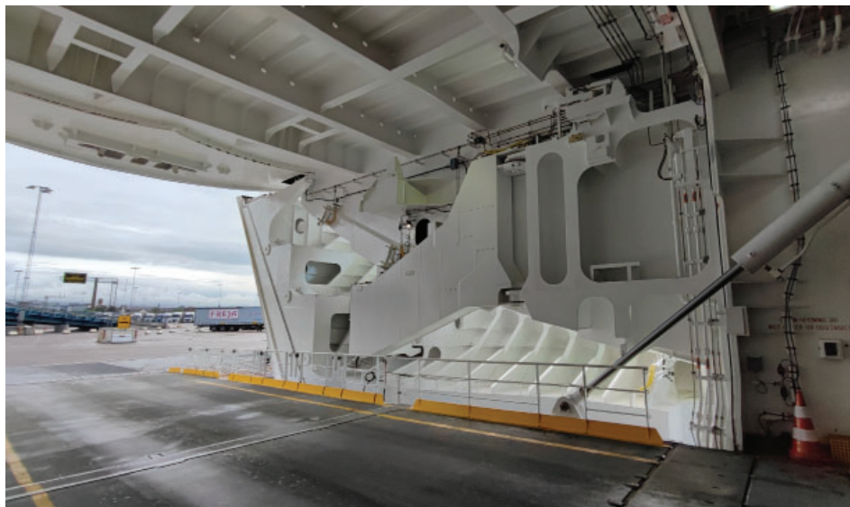
DECK 3 BOW RAMP AND BOW DOOR ARRANGEMENT. SOURCE: PHILIPPE HOLTHOF
